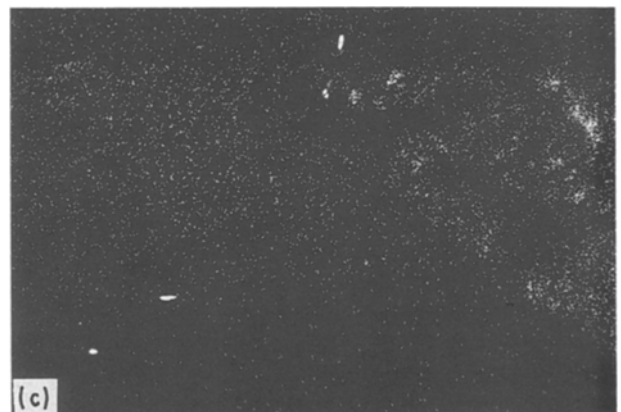
Figure 11 The X-ray map of the transverse section of the precursor film (Sn-5Ti-5Cu wetting on sialon at 1200 K for 20 min, \times 400 ). (a) Sn X-ray map, (b) Ti X-ray map, (c) Cu X-ray map.
